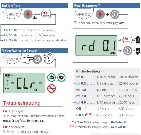
for the display due to electrical malfunction or numerical error. Contact factory for further instructions.
